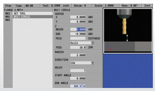
STEP 2 – Select a cycle to be created. In this case, a circular bolt hole pattern.
