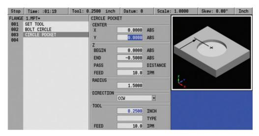
**STEP 4** – Create a second cycle. Adding a circular pocket that is mapped in real time within the help graphic screen.
