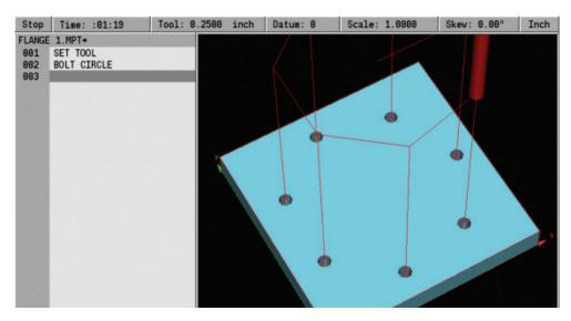
**STEP 3** – Once the circular bolt hole pattern data has been entered into the form press the USE hard key and a graphic of the program is displayed.
