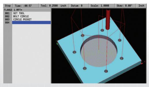
**STEP 5** – Tool paths are also displayed in 3D graphics that can be rotated and manipulated. The program is ready to run. Simply press "GO."
