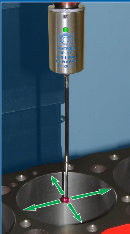
Automatic Part Setup with CNC Probing Cycles*
