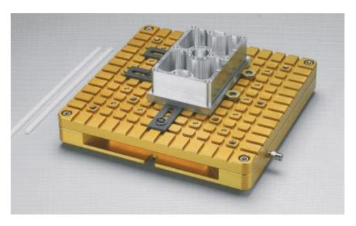
The base and top plate of the Vacu-Vise<sup>™</sup> are constructed of high-grade anodized aluminum with stainless steel fastener hardware. Delrin strips are used for part squaring. For part-holding, foam gasket material fits into the grid matrix channels to create a vacuum seal around the part periphery. Side clamps and Mitee Bites<sup>™</sup> clamps provide an additional holding option.
