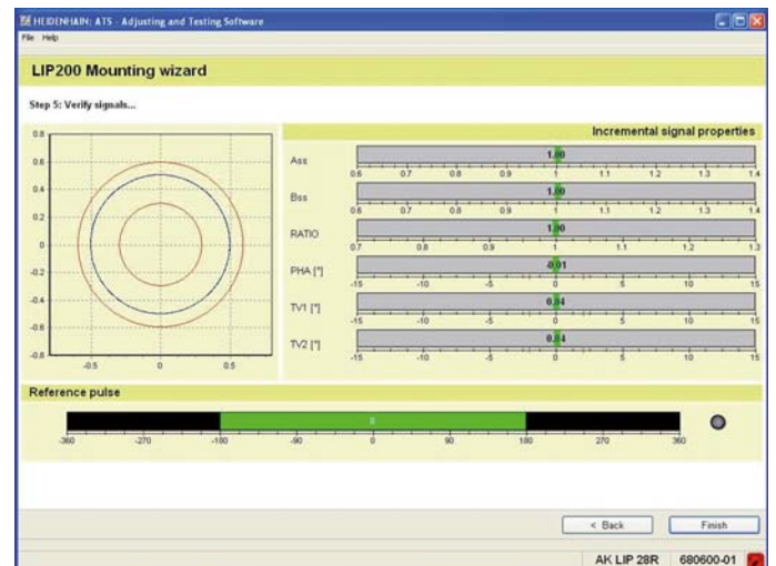
Commissioning using PWM 20 and ATS software
