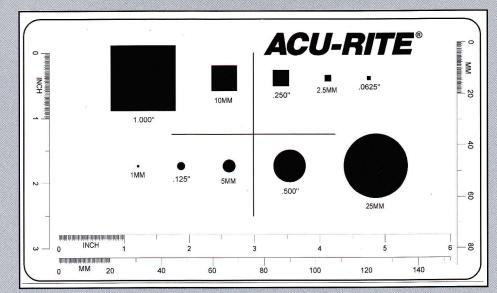
Note: These one inch and 20 millimeter sections are divided into 100 increments. The chrome lines are too fine to represent on paper.
